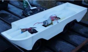
Views showing work so far and the tight curves of the "bow" section, front bumper! Also, for those newbies, note the pink aerial protector used just above the frequency flag 875, compulsory on any radio sets with long aerials, notably 40 and 27 MHz sets. Yes some of these sets are still used by members.
